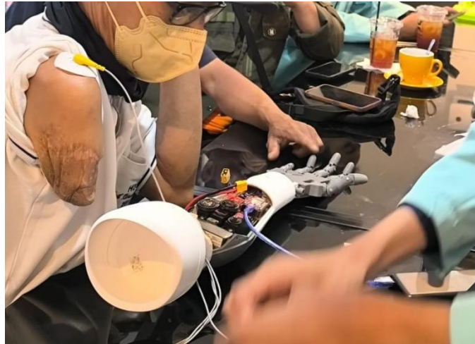
Fig.1 3D-printed prosthetic hand results based on the InMoov design
