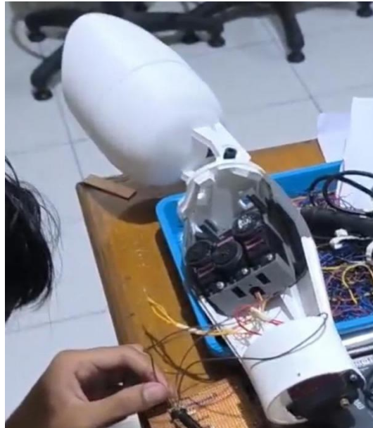
Fig. 4 3D-printed result using PLA filament based on InMoov design
